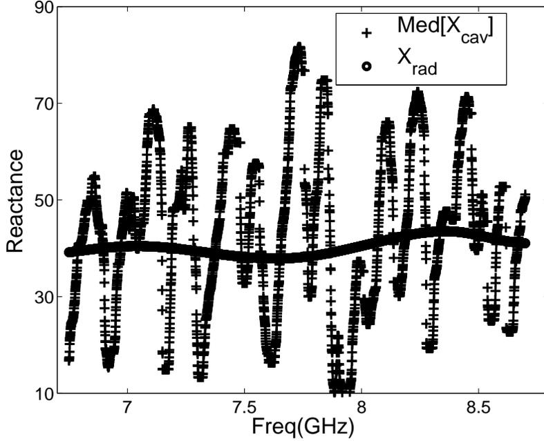
FIG. 5: Median cavity reactance averaged over 100 realization vs. frequencies ranged from 6.75GHz to 8.75GHz, compared with the corresponding radiation reactance  $Im[Z_R(\omega)]$ .
