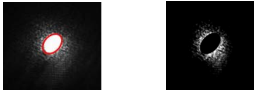
Figure 1: Left: picture of HeNe laser imaged onto a DMA with a defined core specified by the red oval overlay; right: same picture with core light removed.
